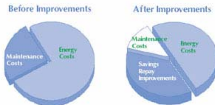
Figure 13. Graphical Representation of How an ESPC Project Is Financed
