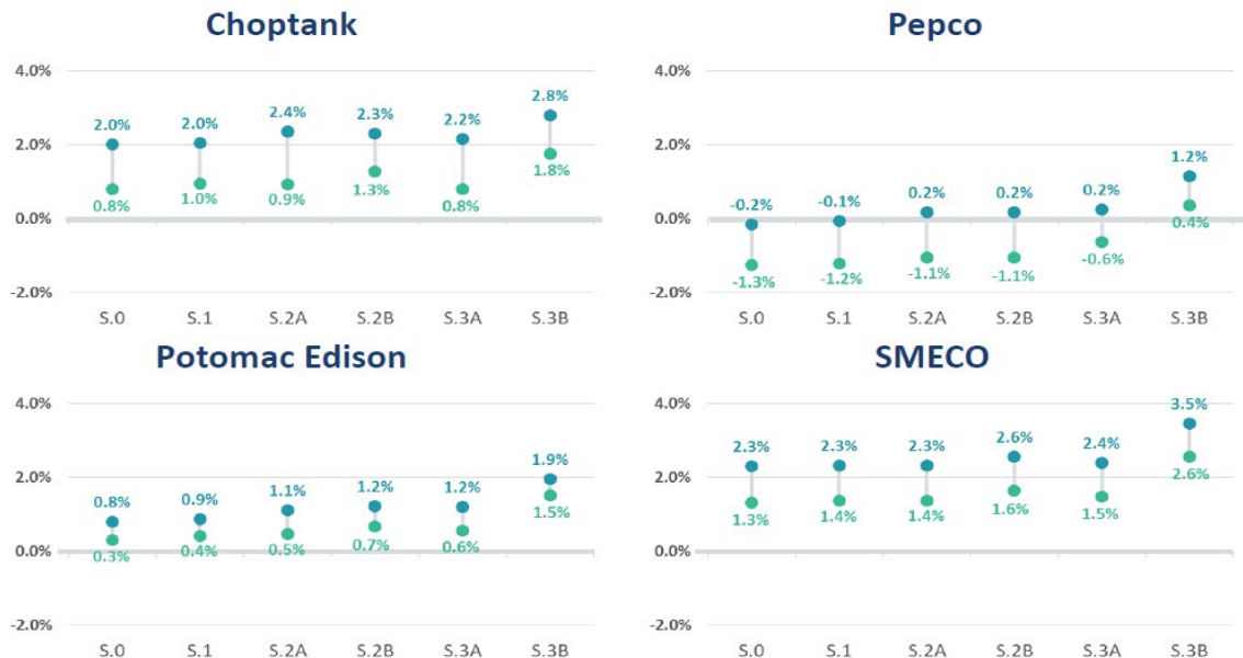
11 Figure 3. 2022–2031 annual peak load growth rate by scenario for selected 12 Maryland utilities
