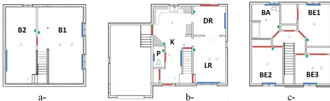
Figure 2. Room layout for a- basement, b- main and c- top floors. Closed doors are shown in red, baseboards heaters in blue and LVCTs locations in green.
